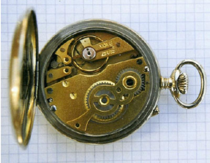
**Fig. 3:** A typical Roskopf movement. But not a trace of Roskopfs trademark. On the plate of the face-side stamped "Swiss".
