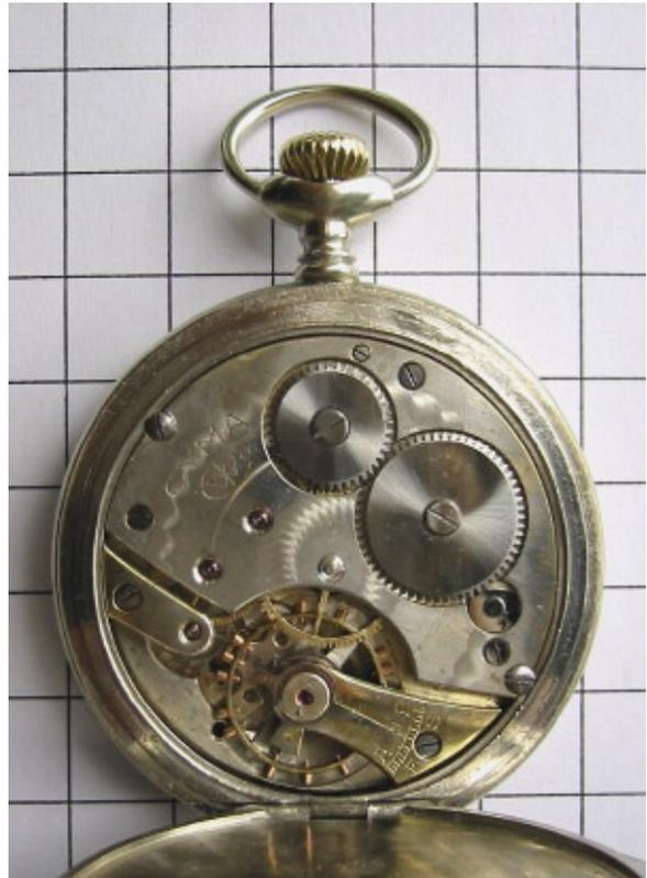
**Fig. 4 + 5:** The Cyma watch with argentan case, silver dial with Braille numerals and gold-plated hands from brass. The pendant shows significant wear by the watch chain, indicating extended use. The watch was overhauled by the author and is in good shape. Watch shown on a 10 millimeter grid.
